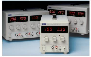
Specifications for Main Outputs: Line & load regulation <0.01%. Output noise <1mV rms. Meter accuracies  $0.3\% \pm 1$  digit - voltage,  $0.6\% \pm 1$  digit - current.
